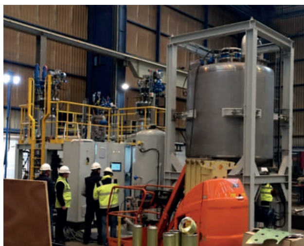
Figure 15: Hydrothermal oxidation demonstrator produced by Leroux & Lotz Technologies as part of the Leanships H2020 project.
