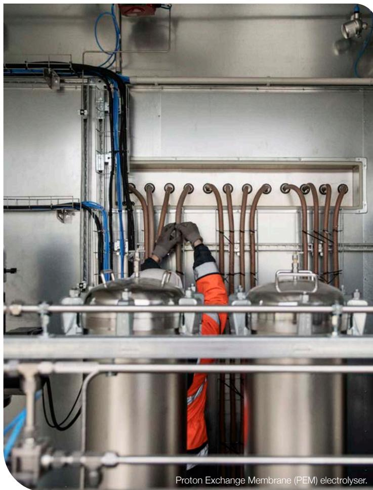
Proton Exchange Membrane (PEM) electrolyser.
